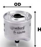
**H** = 125 mm**OD** = 96 mm**IN** = 24.9 mm**OUT** = Special**DRAIN** = 7.1 mm
