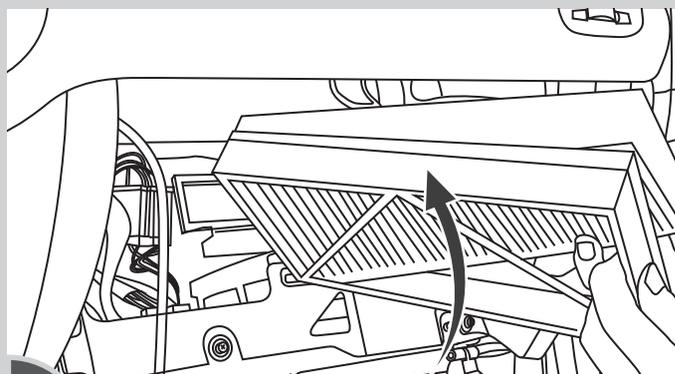
**6** REEMPLAZAR FILTROS EN SUS SOPORTES Y REINSTALAR POR EL PROCEDIMIENTO INVERSO
