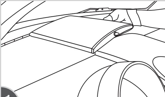
**1** HALAR Y RETIRAR LA CUBIERTA CENTRAL DEL PANEL
